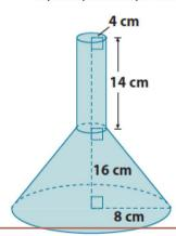
The expression  $\pi 4^2(14)$  represents the volume of the cylinder. The expression  $\left(\frac{1}{3}\pi 8^2(x+16)-\frac{1}{3}\pi 4^2(x)\right)$  represents the volume of the truncated cone. The x represents the unknown height of the smaller cone. When the volume of the cylinder is added to the volume of the truncated cone, then we will have the volume of the funnel shown.
