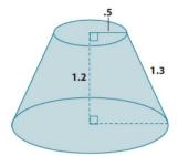
The part of the radius of the bottom base found by the Pythagorean Theorem is 0.5. When we add the length of the upper radius (because if you translate along the height of the truncated cone then it is equal to the remaining part of the lower base), then the radius of the lower base is 1.
